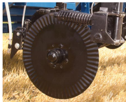
New minimum maintenance coulters design! Totally greaseless hub & frame, Patent Pending.
