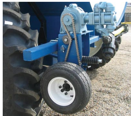
Hydraulic actuated press wheel drive single or twin piston pump. Adjustable drive wheel tension.
